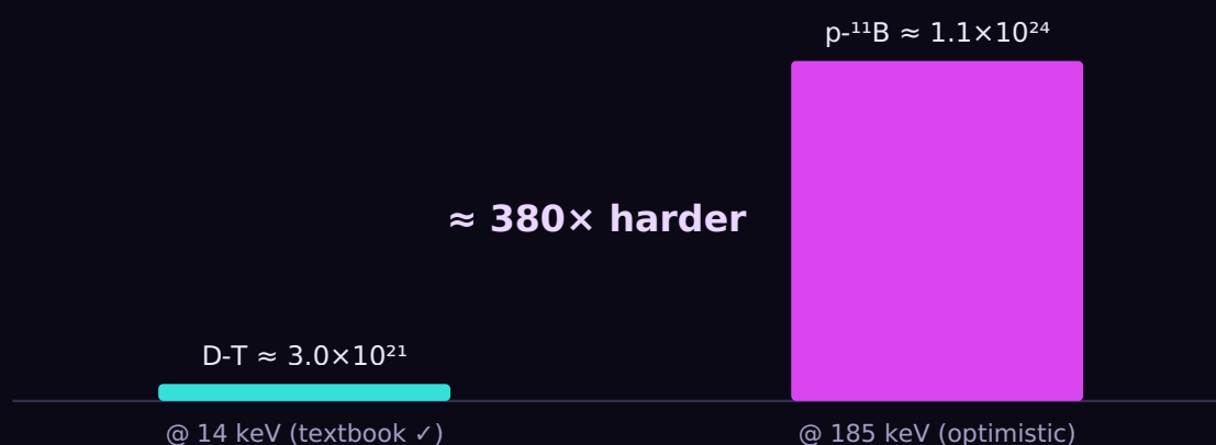
Figure 4 – Ignition-class Lawson requirement (FusionSim v0.3). The D-T minimum reproduces the textbook \sim 3\times 10^{21} \text{ m}^{-3}\cdot\text{keV}\cdot\text{s} , validating the method; p\text{-}^{11}\text{B} is \sim 380\times harder even under optimistic assumptions. Reproducible: FusionSim v0.3 Lawson module.
